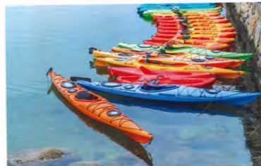
▲ Canoes made from moulded GRP
